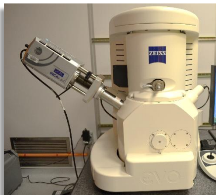
Zeiss EVO Environmental SEM
