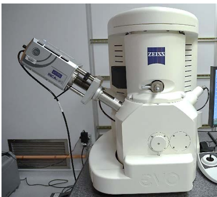
Zeiss EVO Environmental SEM
